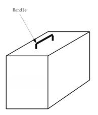
For MMA- series (discrete) arc welding machine, the handles are installed at the top of machine to move it. The machine needs immobile equipment to fix to avoid sliding.
