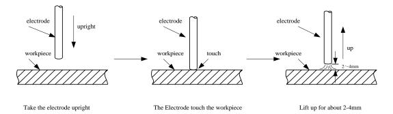
Lifting arc: take the electrode to scrape the workpiece for striking arc. But it may cause the arc scratch, so must to lift arc in the groove.
