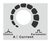
Adjustment knob position multi circle potentiometer, next to no mark the specific welding current value size, clockwise rotation set value increased.
